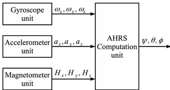
Fig. 1. The block-diagram of attitude and heading reference system
