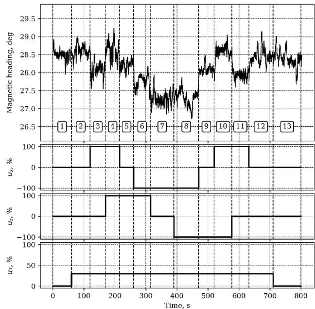
Fig.5. Experiment results:  $U_x$  is a signal of the longitudinal control;  $U_z$  is a signal of the lateral control;  $U_t$  is a signal of motor trust
