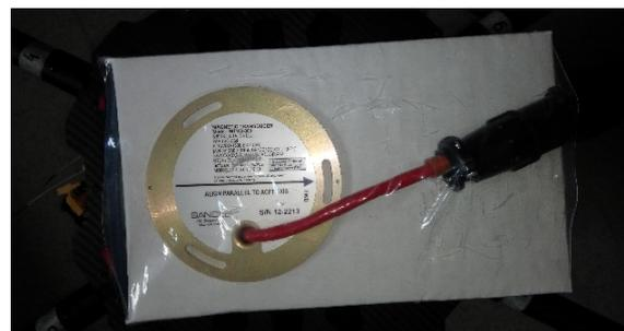
Fig. 3. Attitude and heading reference system
