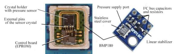
Fig. 2. Pressure sensor BMP180
