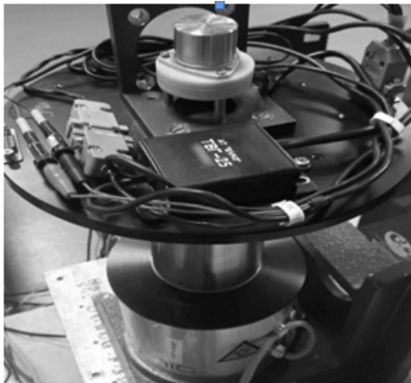
Fig. 6. Metallic resonator CVG mounted on a turntable to calibrate during rotation
