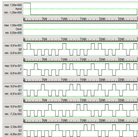
Fig. 8. Waveforms of nanoregister operation (Galois configuration)
