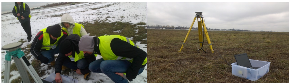
Fig. 4. Measurement equipment adjustment and GNSS data recording
