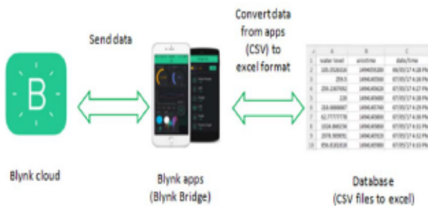
Fig. 4. The flow of database via Blynk application
