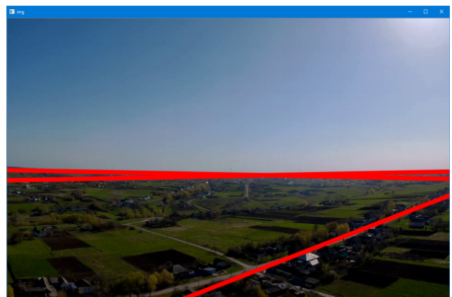
Fig. 5. Received determination of the main road (horizon line is detected as landmark)
