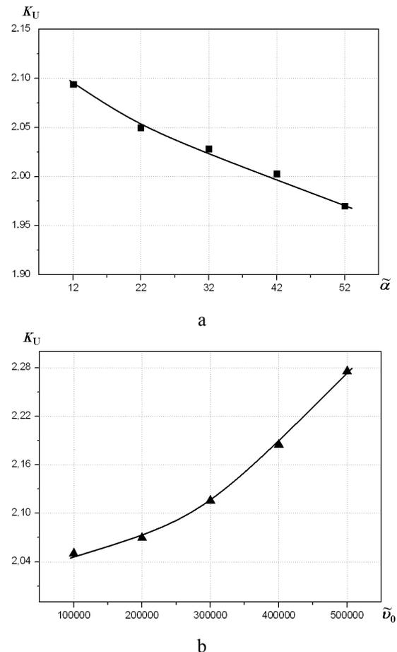
Fig. 1. Theoretical dependences  $K_U$  change at ascending of CM machining speed (a) and ascending parameter characterizing CM physical-mechanical characteristics (b)
