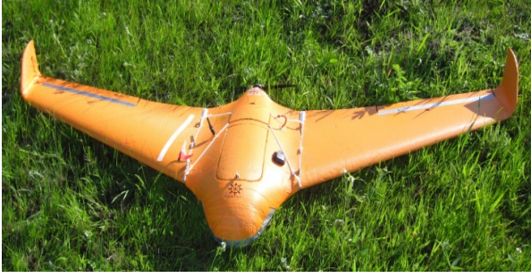
Fig. 1. Skywalker X8 flying wing with the mini autopilot developed in at the National Aerospace University (KhAI) in Kharkov, Ukraine
