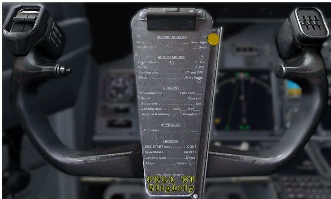
Fig. 5. Indication of the alarm trigger warning of preventing sharp movements on the steering wheel
