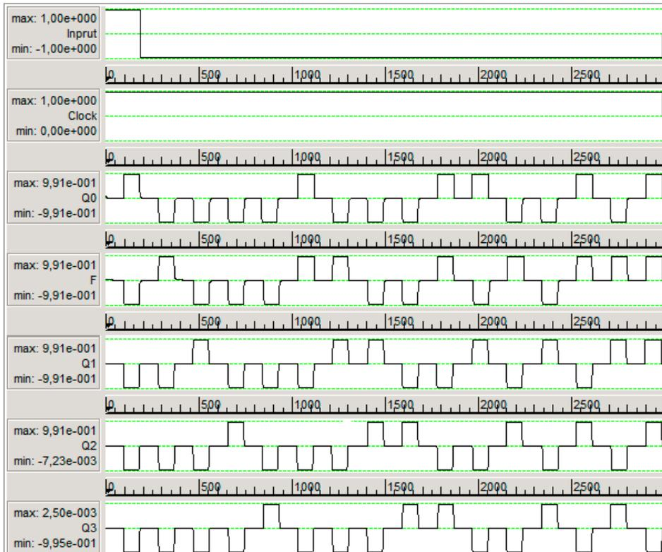
Fig. 8. Time diagram of nano-register operation
