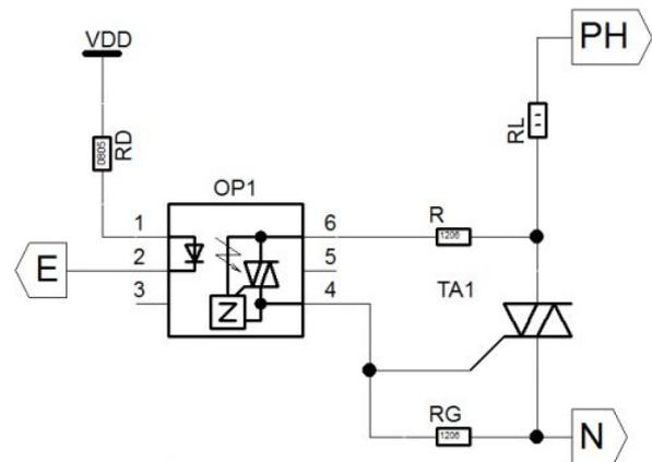
Fig. 3. Schematic realization of the power switch
