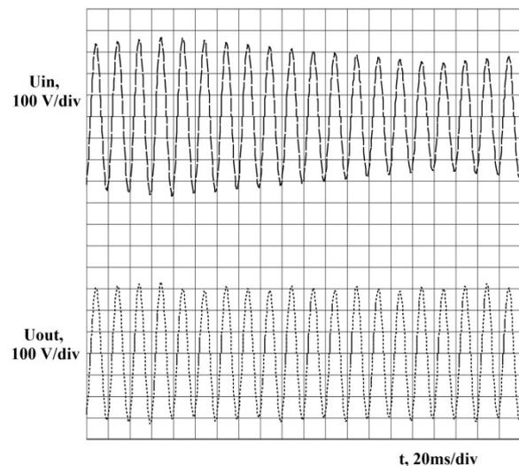
Fig. 5. Time diagrams of the input and output voltages
