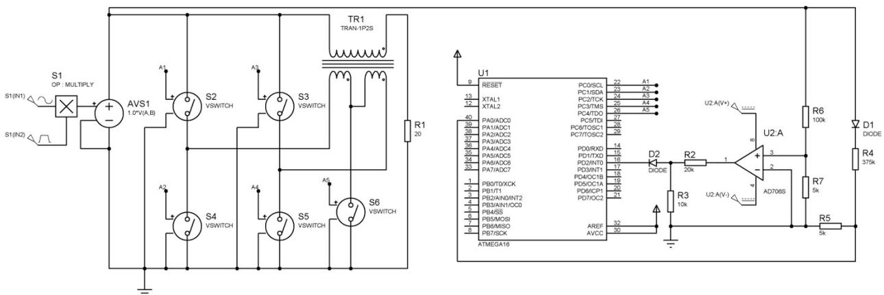
Fig. 4. Virtual model of discrete voltage stabilizer with control system
