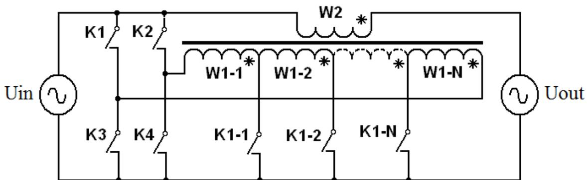
Fig. 1. Structure of the discrete voltage stabilizer
