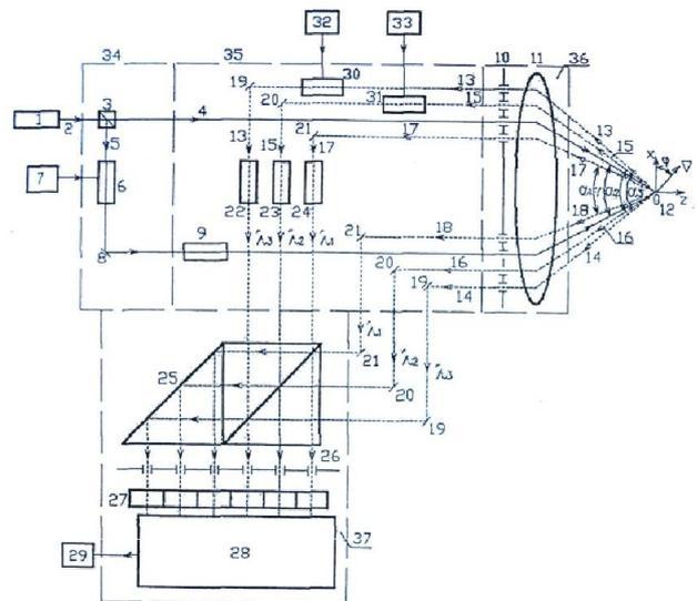
Fig. 3. Multiwavelength laser doppler anemometer (MLDA)
