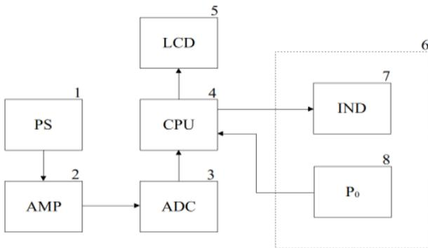
Fig. 4. Barometric Altimeter scheme: 1 is the pressure sensor; 2 is the amplifier; 3 is the analog to digital converter; 4 is the microcontroller; 5 is the liquid crystal display; 6 is the PC software; 7 is the indicator; 8 is the ground pressure setter
