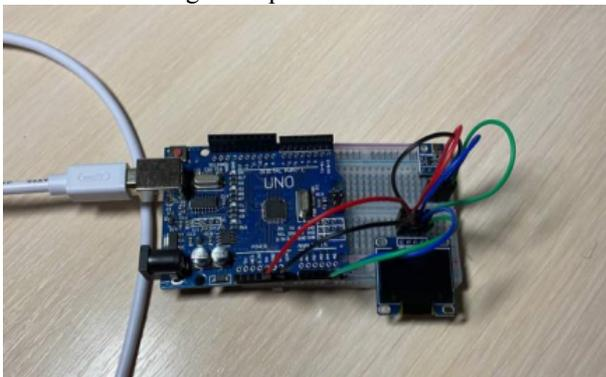
Fig. 5. Assembled MEMS Barometric Altimeter
