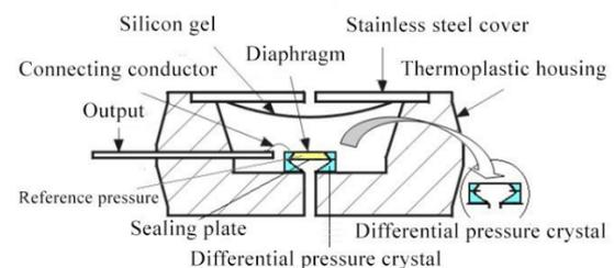
Fig. 1. Basic housing of the pressure sensor
