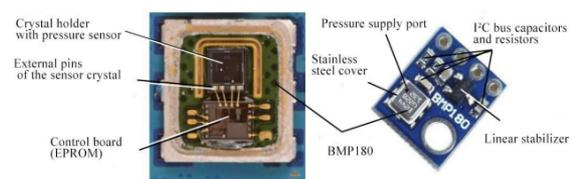
Fig. 2. Pressure sensor BMP180
