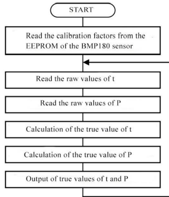
Fig. 3. Principle of work BMP180
