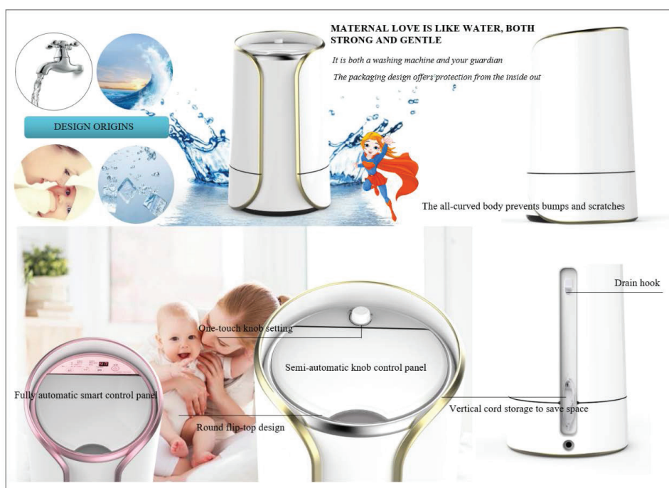
Fig. 4. Design concept of mini washing machine for mother and baby (Drawn by the author)
