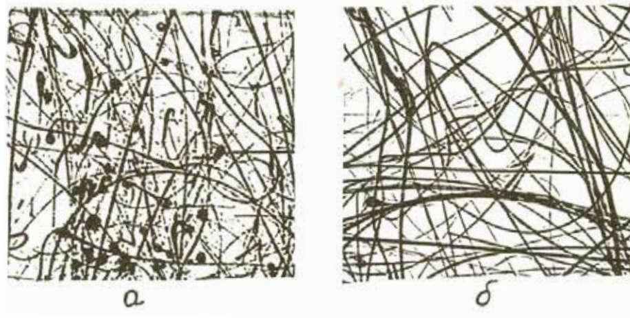
Fig. 6. Structure of Microfine Basalt Fibers
