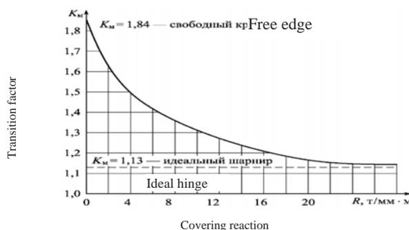
Fig. 1. Butt joint rigidity impact on the pavement bearing capacity
