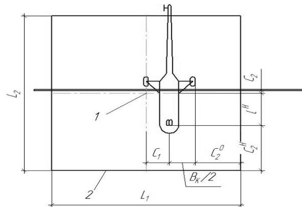
Fig. 5. Scheme for determining the size of helicopter landing sites:
