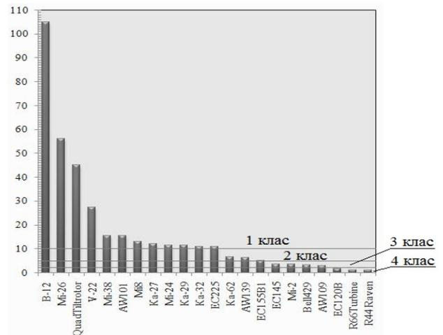
Fig. 8. Helicopters classification by take-off weight according to the ICAO
