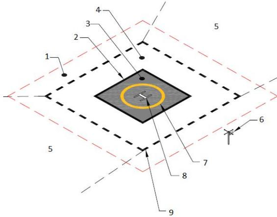
Fig. 4. The main parts of the landing site [7]:
