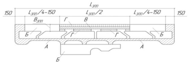
Fig. 7. The scheme of airfield pavement division into groups of sections:
