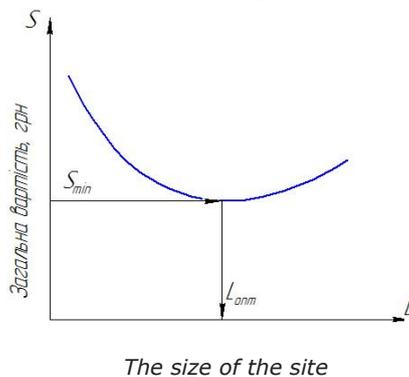
Fig. 6. Dependence of the total cost of construction on the size of the site
