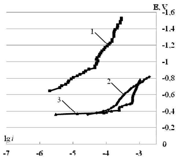
**Fig. 2.** Potentiostatic polarization curves in 0,5 mol/l solutions of isovaleric aldehyde (25 °C): 1 – aluminum in aqueous – alcoholic solution of 10 g/l  $\text{Na}_2\text{SO}_4$  (pH = 7,98), 2 – aluminum and 3 – cadmium electrodes in sulfuric acid-aqueous-alcohol solution (pH = 2,98)
