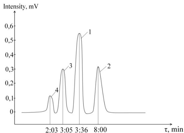
**Fig. 3.** The chromatogram of electroreduction products of isovaleric aldehyde in sulfuric acid-aqueous-alcohol solution under regular controlled potential ( $E = -0,7\text{V}$ ): 1 – isopropyl alcohol (solvent), 2 – isovaleric aldehyde, 3 – isopentane, 4 – isopenten
