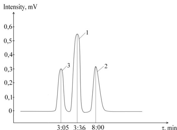
**Fig. 4.** The chromatogram of electroreduction products of isovaleric aldehyde in sulfuric acid-aqueous-alcohol solution under regular controlled potential ( $E = -0,75\text{V}$ ): 1 – isopropyl alcohol (solvent), 2 – isovaleric aldehyde, 3 – isopentane
