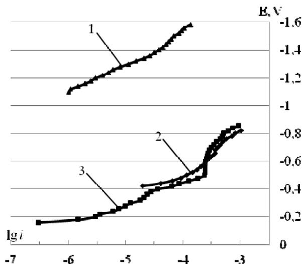
**Fig. 1.** Potentiostatic polarization curves of metals (25 °C): 1 – aluminum in aqueous-alcohol solution of 10 g/l  $\text{Na}_2\text{SO}_4$  (pH = 7,98), 2 – aluminum – and 3 cadmium in sulfuric acid-aqueous-alcohol solution (pH = 2,98)
