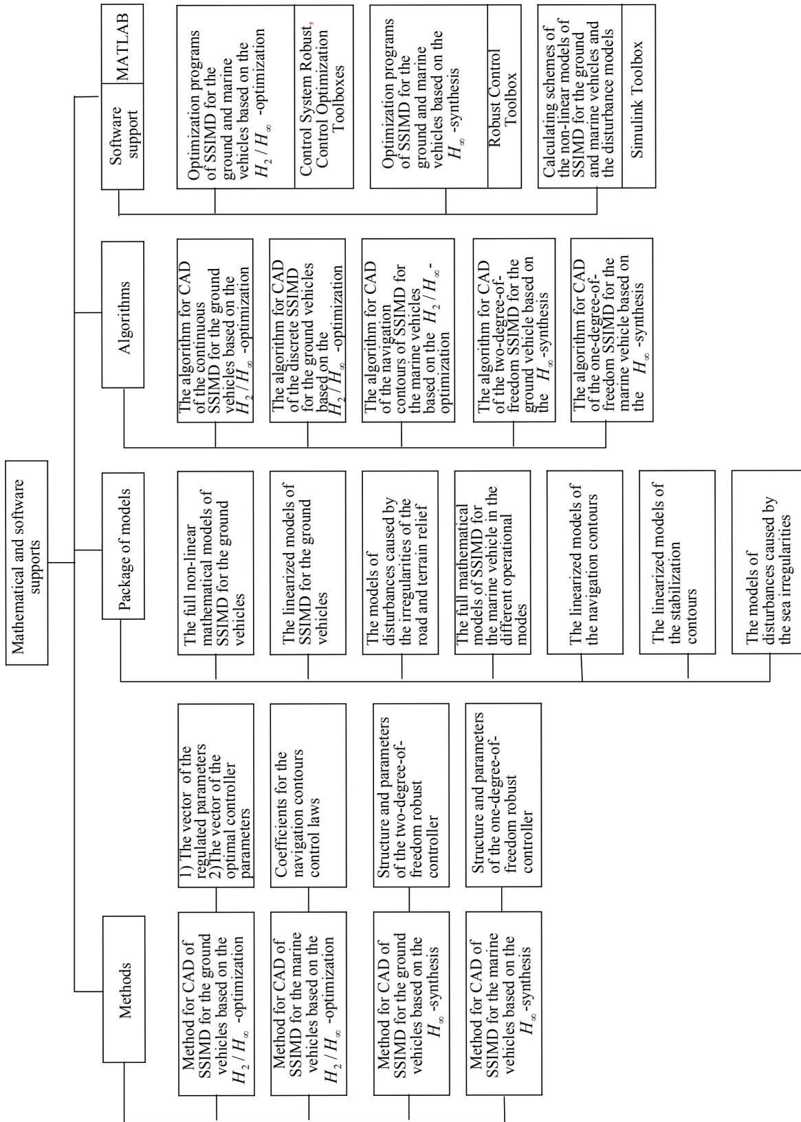
**Fig. 1.** The mathematical and software support of the CAD system for the SSIMD design: CAD – computer-aided design; SSIMD – system of stabilization for information-measuring devices
