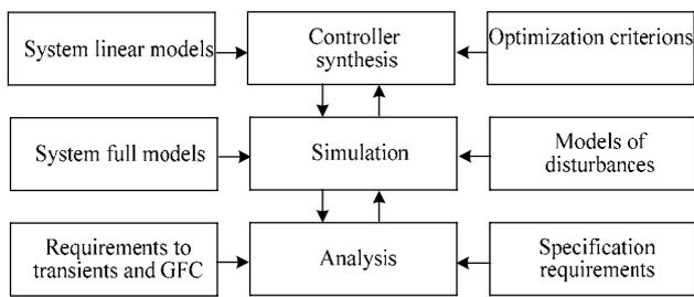
**Fig. 5.** Design of the robust regulator:
