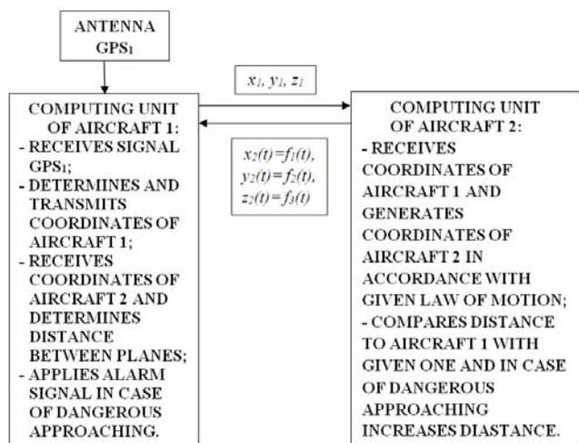
Fig. 4. Scheme of simulation of aircraft approaching
