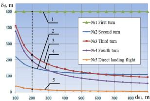
Fig. 4. Dependency graph of the error determining, by the MPLS system, the aircraft deviation from the center line of the runway at turns and on the aircraft direct flight trajectory  $\delta_d$  versus the distance between its GE components  $d_{01}$
