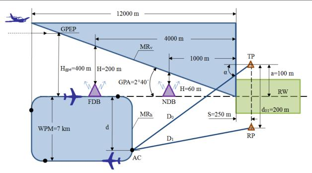
Fig. 3. The basic geometric correlation between the placement of beacons and runway to the estimation of errors in determining AL during its pre-landing maneuvering
