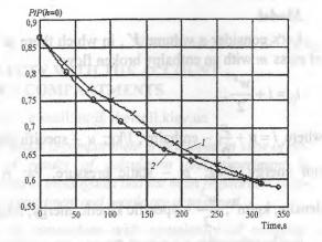
Fig. 1. Comparative estimation of results of calculation and experiment of air pressure variation in a compartment P/P(h = 0) concerning a standard atmosphere with respect to the time: I – experiment; 2 – calculation
