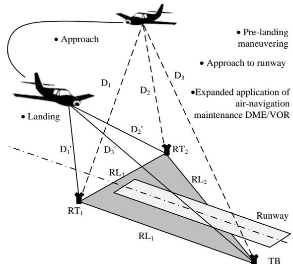
Fig. MPLS operating principle
