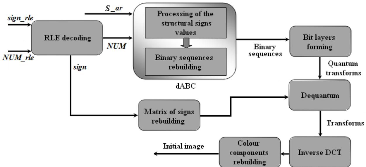
Fig. 3. Structural scheme of the improved algorithm of proceeding of images on the base of the method of dABC
