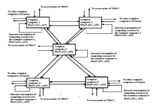
Fig. 2. Fully connected cluster with five complete computers
