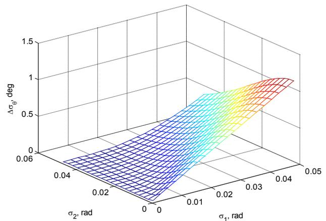
Fig. 3. Attitude error difference between the TRIAD and the QUEST methods
