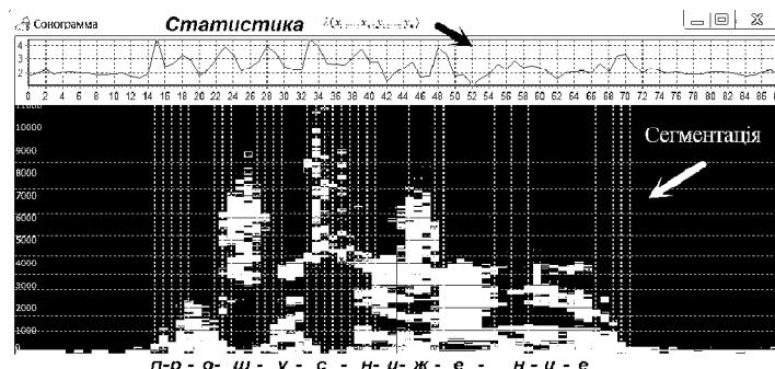
Fig. 2. Segmentation's result on phrase «Прошу снижение» (on Russian). Top chart show values of statistic  $\lambda$ . Vertical dotted lines shows the moments of phoneme changes
