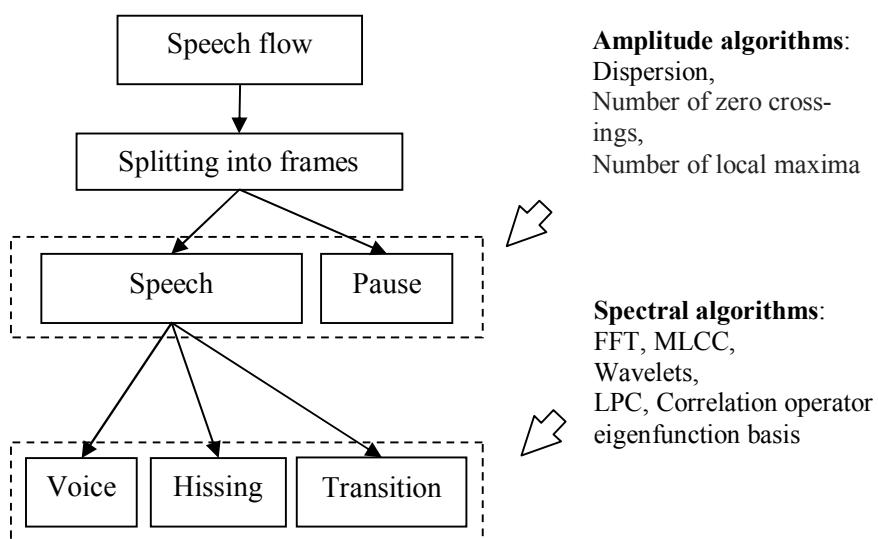
Fig. 1. Classification of segmentation algorithms
